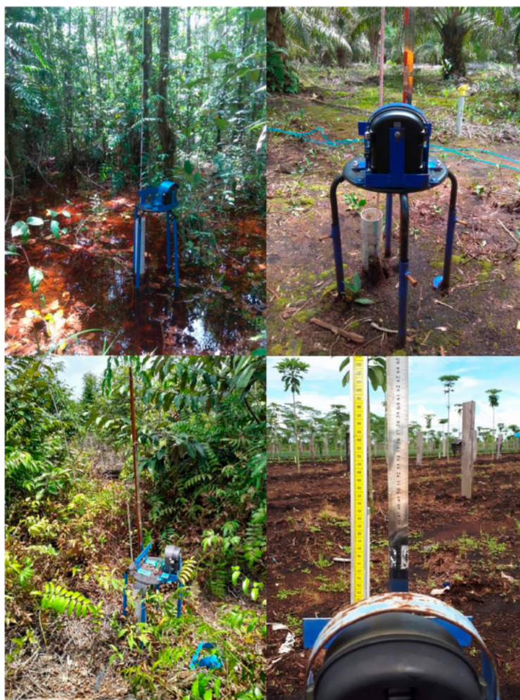
FIGURE 2 | Peat cameras installed at four sites in Central Kalimantan (clockwise from top left: Forest, oil palm plantation, smallholder agriculture, previously burned scrubland).
